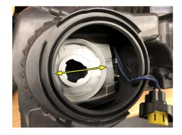
With the bulb socket opening moved down you can now insert the G11 Series bulb and twist it into place.
